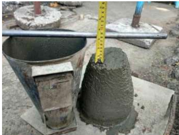
Figure 4: Determination of the slump
