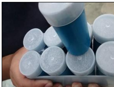
Fig. 1.28: Exothermic black powder used in the Cadweld process
