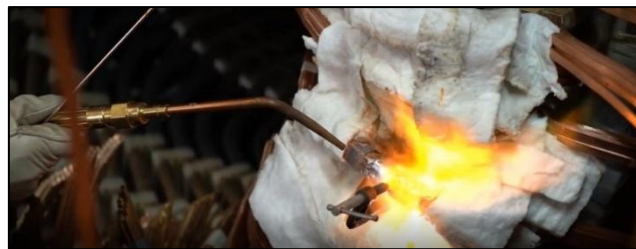
Fig. 1.30: Oxy-acetylene brazing/welding applied during the manufacture of large industrial motors.
