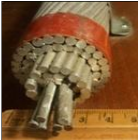
Fig. 3: The conductor consists of seven strands of steel surrounded by four layers of aluminum
